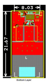
Figure 31. Recommended PCB Layout
