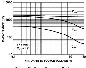
Figure 21. Capacitance vs Drain to Source Voltage
