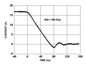
Figure 27. FDMS3669S SyncFET<sup>TM</sup> body diode reverse recovery characteristic
