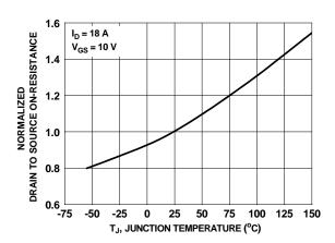
Figure 16. Normalized On-Resistance vs Junction Temperature
