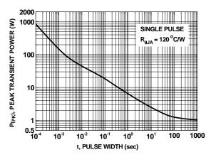
Figure 25. Single Pulse Maximum Power Dissipation
