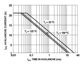
Figure 9. Unclamped Inductive Switching Capability
