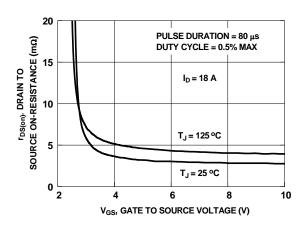
Figure 17. On-Resistance vs Gate to Source Voltage
