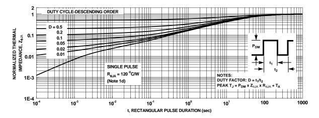
Figure 26. Junction-to-Ambient Transient Thermal Response Curve
