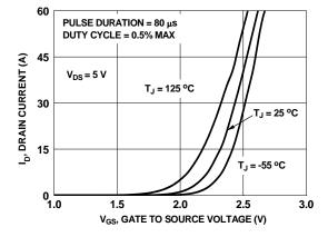
Figure 18. Transfer Characteristics
