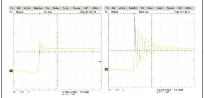
Figure 29. Power Stage phase node rising edge, High Side Turn on
