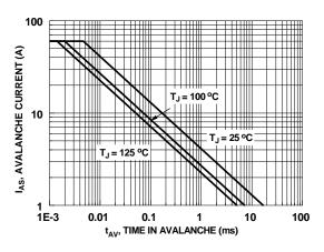
Figure 22. Unclamped Inductive Switching Capability
