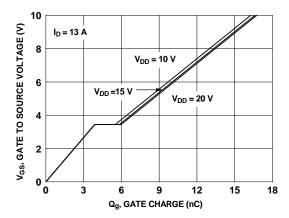
Figure 7. Gate Charge Characteristics
