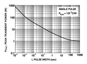
Figure 12. Single Pulse Maximum Power Dissipation
