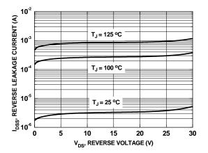
Figure 28. SyncFET<sup>TM</sup> body diode reverse leakage versus drain-source voltage
