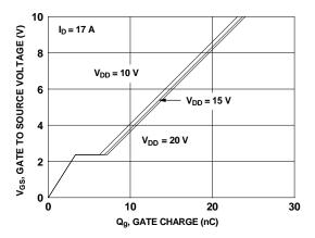
Figure 20. Gate Charge Characteristics
