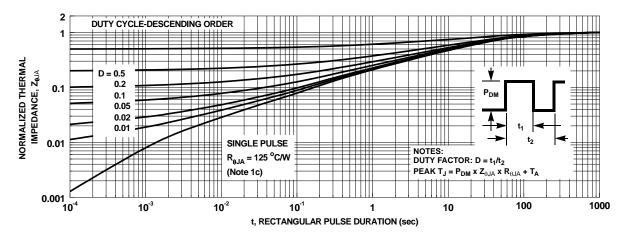
Figure 13. Junction-to-Ambient Transient Thermal Response Curve
