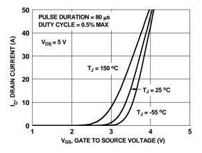
Figure 5. Transfer Characteristics
